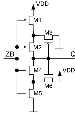
Figure 5. Schmitt Trigger CMOS circuit
