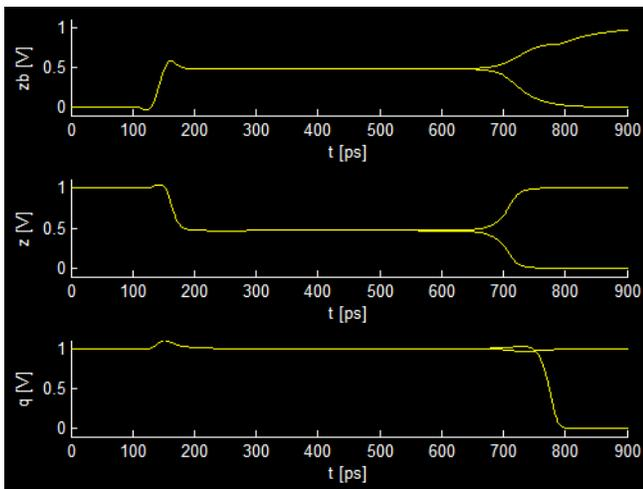
Figure 7. Simulation result for the van-Berke implementation with the Schmitt-Trigger output stage (inverting loop node starting low)
