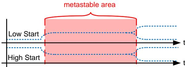
Figure 1. Metastability behavior of a storage loop (inverting node)
