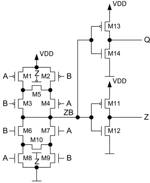
Figure 3. Van-Berkel Muller C-element CMOS implementation
