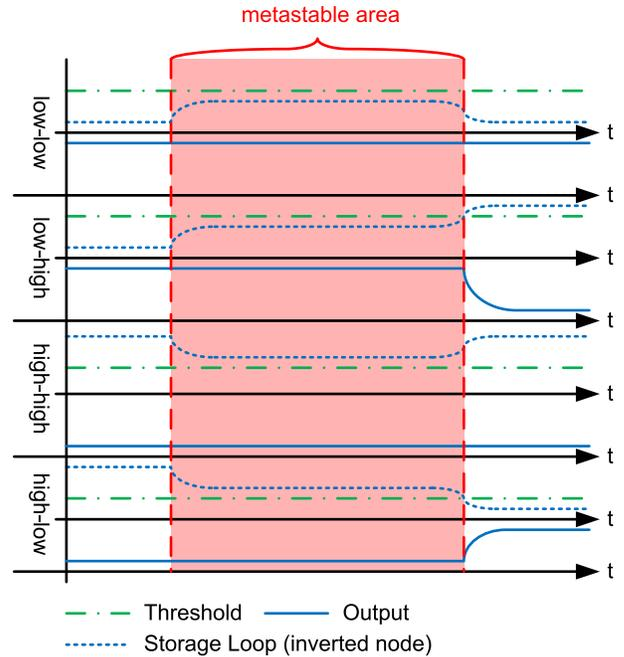
Figure 2. Metastability mitigation principle
