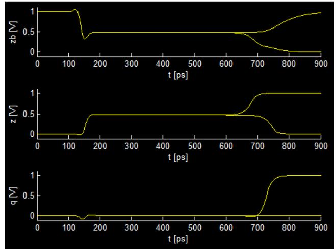
Figure 6. Simulation result for the van-Berkel implementation with the Schmitt-Trigger output stage (inverting loop node starting high)
