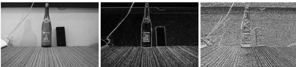
Figure 5: The intensity (left), difference (middle) and orientation (right) values of the pixels of an image
